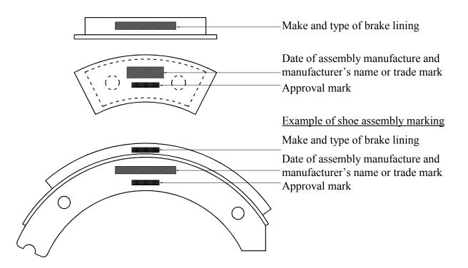
Example of drum brake lining marking
